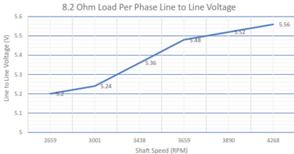
Figure 6: Terminal Voltage with 8.2 Ohm Star-Connected Load
