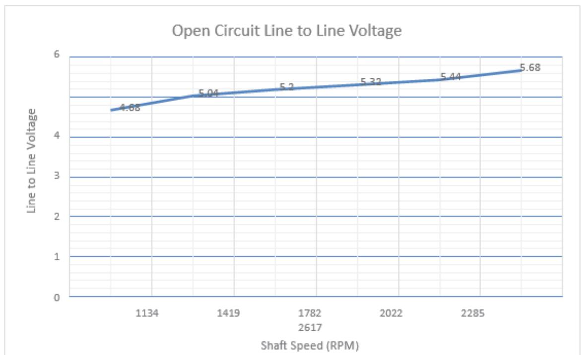
Figure 2: Open Circuit Terminal Voltage at Different Shaft Speeds
